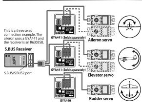
Gyro gain CH(Receiver)←connect→Port2(GYA440)
