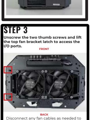
fully remove the top fan bracket.
