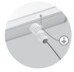
**Note:** For lightning and ESD protection, connect the EAP's grounding terminal to grounding facilities using a proper grounding wire, which should meet local installation requirements.
