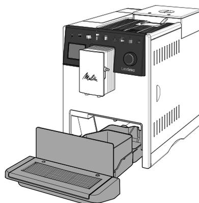
The drip tray can be pulled forwards out of the appliance. Always empty both the drip tray and also the coffee grounds container. Then, make sure you push the drip tray into the appliance up to the stop.
