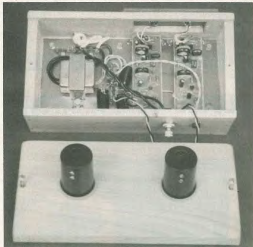
FIG. 7—MOUNT THE MODULES for the stereo transmitter in a cabinet along with the power-supply components or a battery pack if you so desire.
