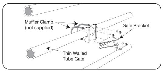
Muffler Clamp for Gate Bracket
