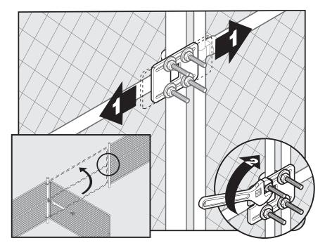
**Note:** For MM372W installations, the closed position stop plate should be installed on the leading edge of the PRIMARY gate leaf, and adjusted to close against the leading edge of the SECONDARY gate leaf (see page 22).
