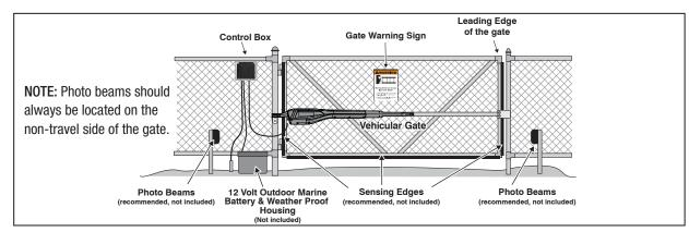
**Example of MM371W Installation** (Installations vary slightly on different types of gates)
