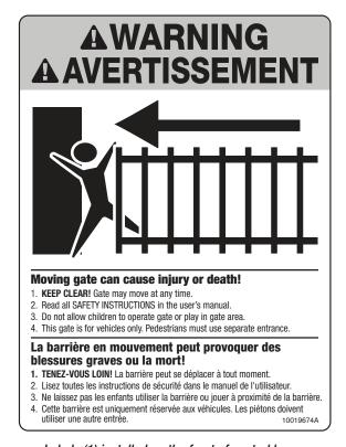
Labels (1) installed on the front of control box
