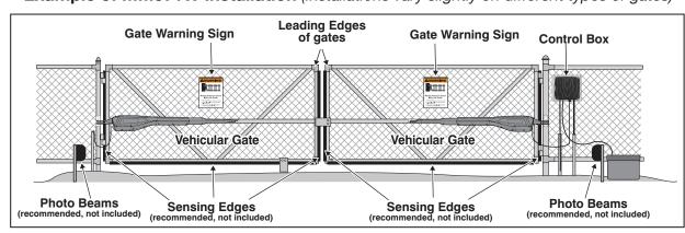
**Example of MM372W Installation** (Installations vary slightly on different types of gates)
