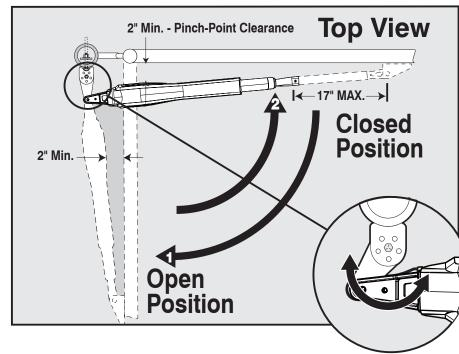
WARNING: ENSURE THE REAR MOUNT DOES NOT MAKE CONTACT WITH THE POST-BRACKET ASSEMBLY DURING ANY POINT OF THE GATE TRAVEL.
