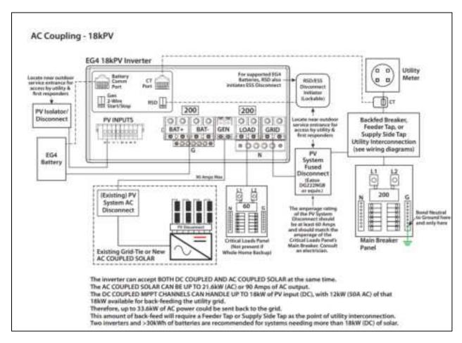
Be sure to follow these steps to avoid configuration errors or wiring issues, which can lead to poor or improper system performance.
