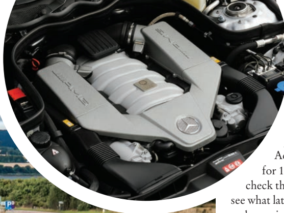
◀ 6.2-litre, naturally aspirated V8 with 518bhp in first E63.
