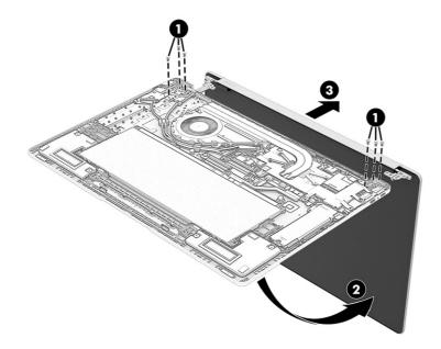
9. (OLED panels) To remove the display bezel from OLED displays:
