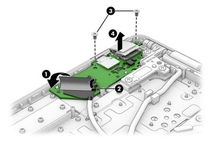
5. To remove the USB door, lift the front of the door up to remove it from the board.
