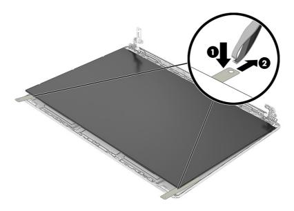
c. Remove the cables (1) from the channel at the bottom of the display.
