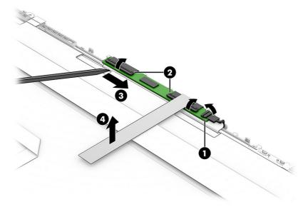
12. (OLED models) To remove the camera module from the back of the display panel on OLED models:
