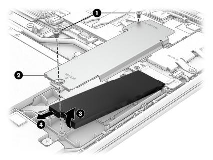
4. When installing an SSD, be sure an undamaged thermal pad is installed on the bottom of the SSD bracket.
