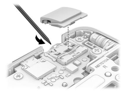
To install the USB/audio board, reverse this procedure.
