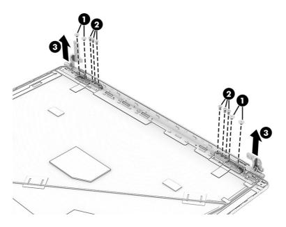
17. To remove the wireless antennas and cables:
