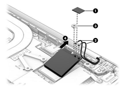
5. If the WLAN antenna is not connected to the terminal on the WLAN module, install a protective sleeve on the antenna connector, as shown in the following illustration.
