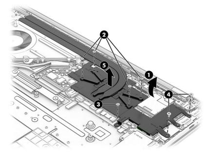
6. Each time the heat sink is removed, thoroughly clean and replace the gray thermal paste (1), and confirm installation of the thermal pads (2) on the heat sink.
