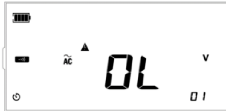
Figure 13.14 The measured AC voltage exceeds the range
