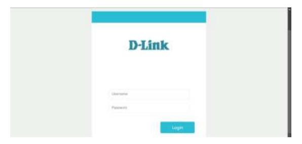
3. If you forget your login password, press and hold the reset button on the back of the router for 5-8 seconds to reset it, and then proceed with the configuration in the previous step.
