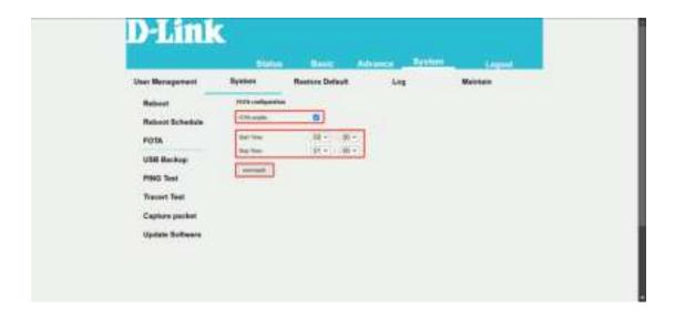
The router will check for new version during each set time period, if a new version is found it will automatically upgrade.
