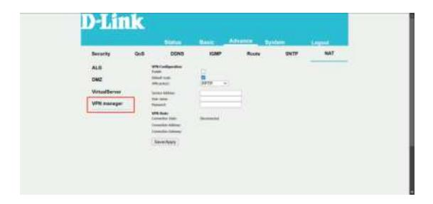
Check the "Enable" option box, choose the "VPN protocl", fill in "Service Address", "User name" and "Password", click "Save/Apply" button.
