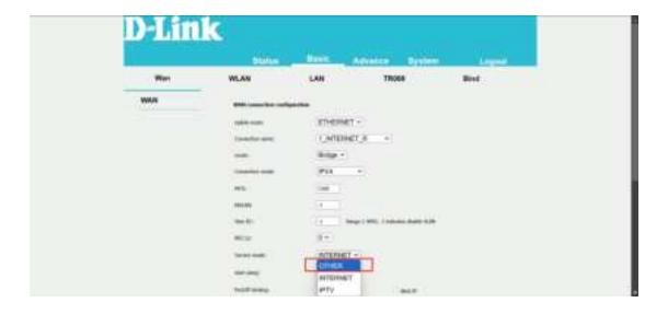
3. Check the LAN port or SSID that needs to be activated, and click "save/apply" to save and make it effective.
