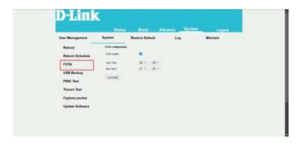
Confirm that the FOTA function is enabled and set the time period for detecting upgrade, click the "save/apply" button to save the configuration.
