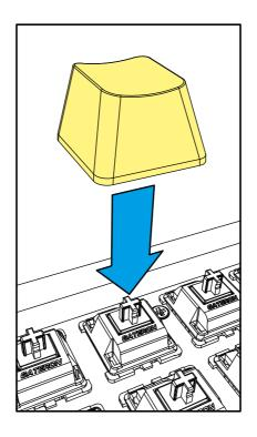
To install a keycap, first place it over the installed switch. Make sure that the keycap's symbol or character is positioned the right way round. Now carefully press the keycap onto the switch until the keycap locks into place. Do not use excessive force, as this can damage the keycap and the switch! After the correct installation, the switch and keycap should behave as when used for normal typing.
