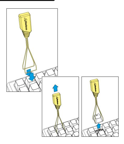
To remove a keycap, place the arms of the keycap puller tool either to the left and right or to the top and bottom of the keycap, and then pull the keycap upwards with careful but constant pressure. Whenever possible, avoid pulling the keycaps from the switch directly with your fingers, as this may damage the switch.
