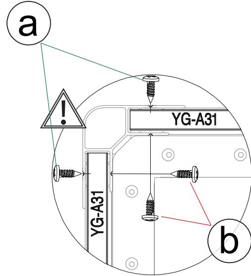
Ensure the panels are fully inserted into the slots to avoid issues with inserting subsequent panels.
