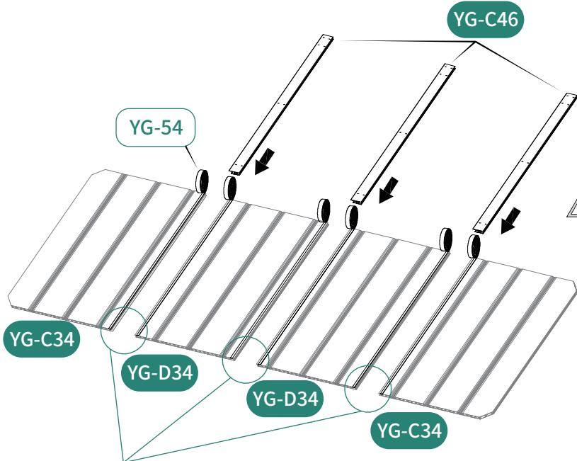
Attention, the screws should be fixed in the waterproof rubber/sealant section.
