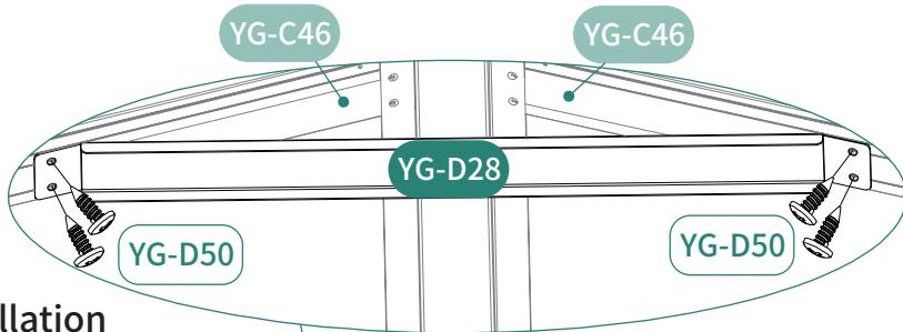
Undertake the installation process by accessing it from the roof's inner space/interior.
