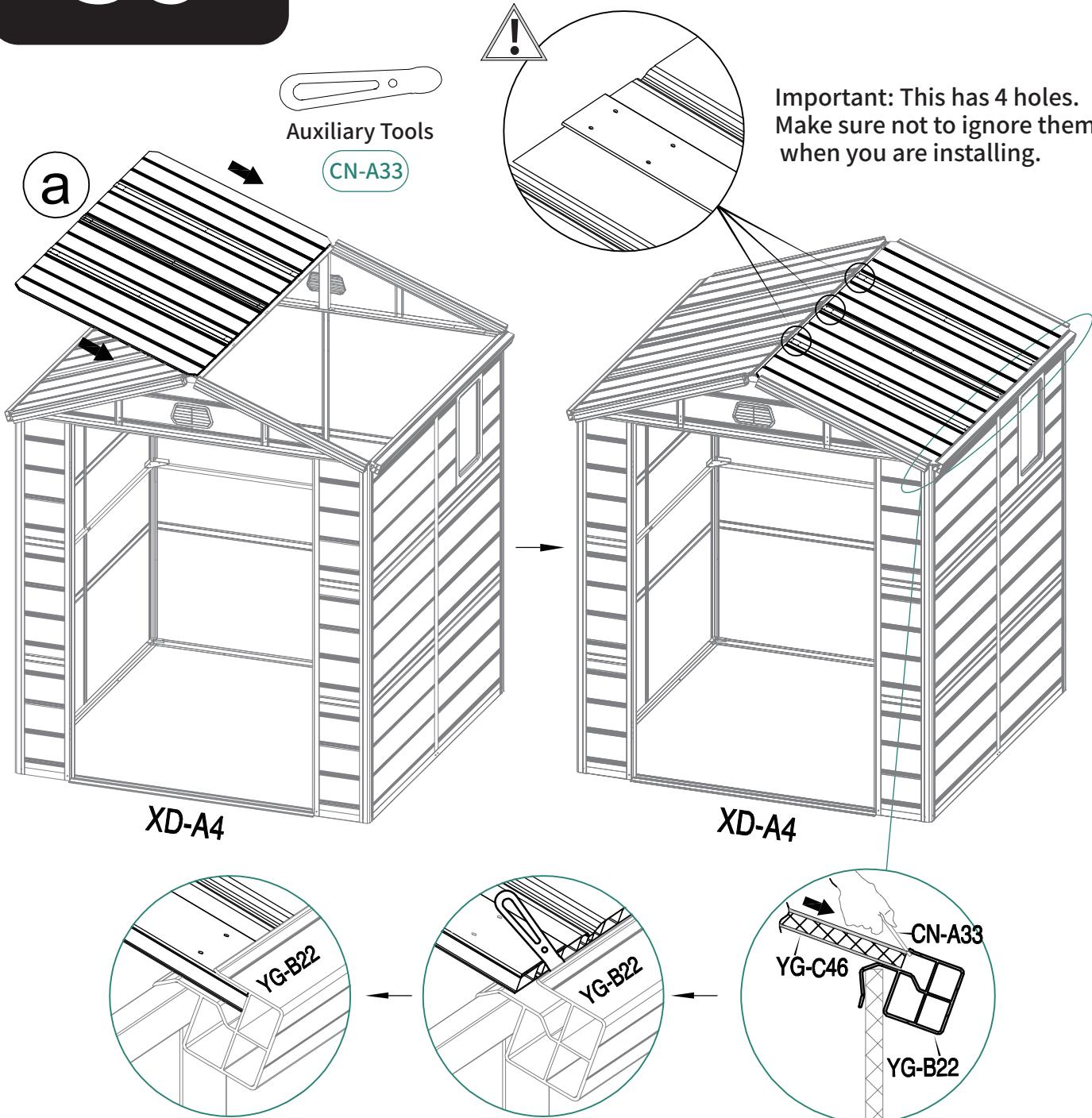
When sliding the roof panels into the slots, please use an assisting tool to ensure they are fully inserted into the tracks.
