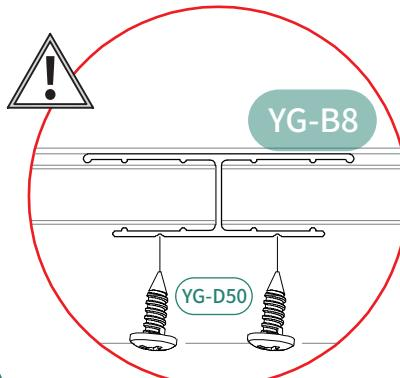
After the panel is installed, secure it from the inside using screws. When fastening, please align the screws with the grooves to avoid any deviations that could lead to loosening.
