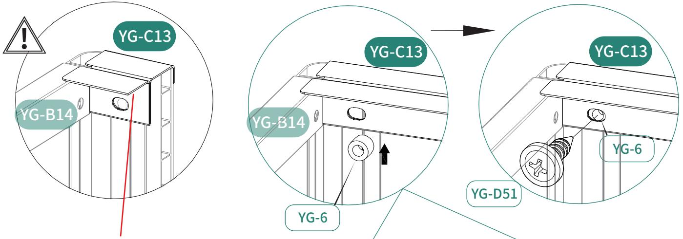
Ensure the folded edge of the component is facing inwards.
