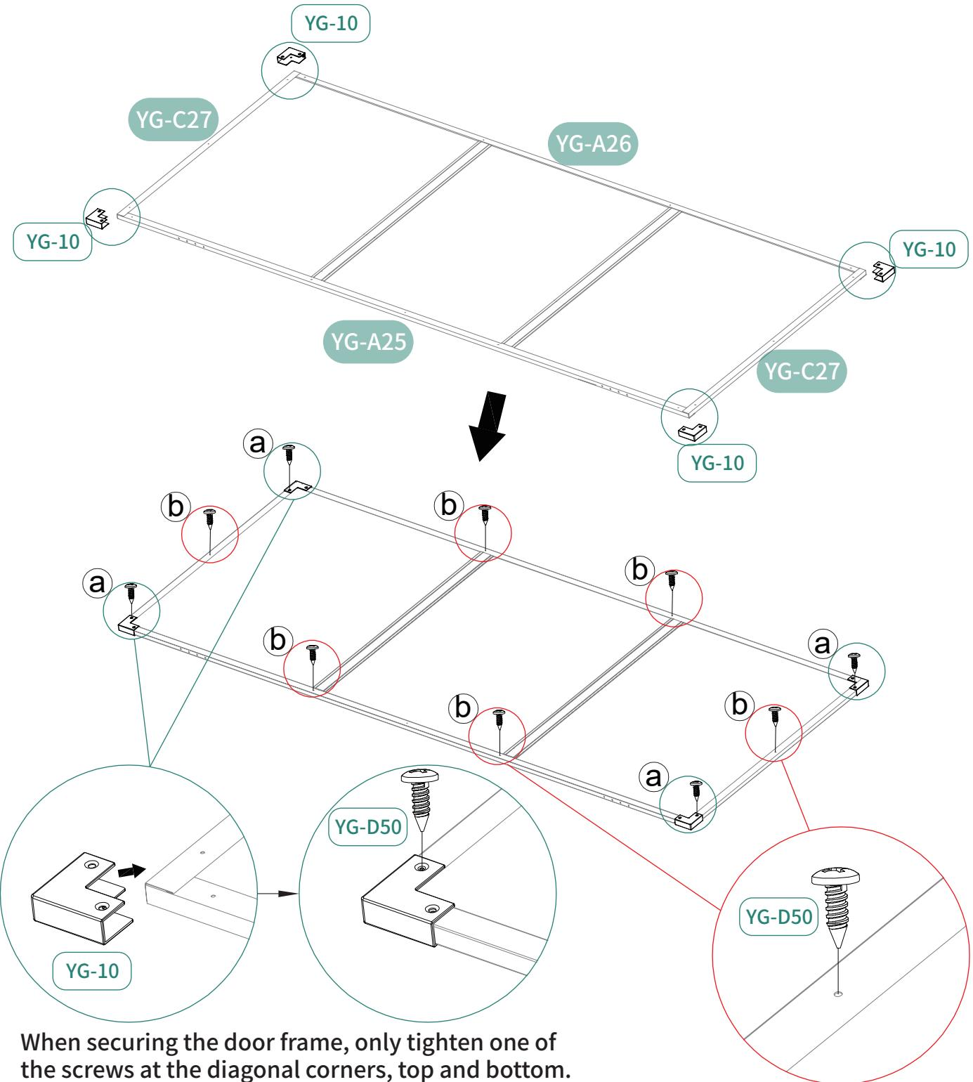
When securing the door frame, only tighten one of the screws at the diagonal corners, top and bottom.
