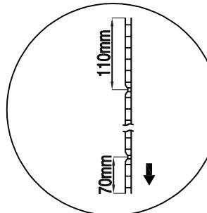
During installation, ensure the narrow edge of the panel is oriented facing downward.
