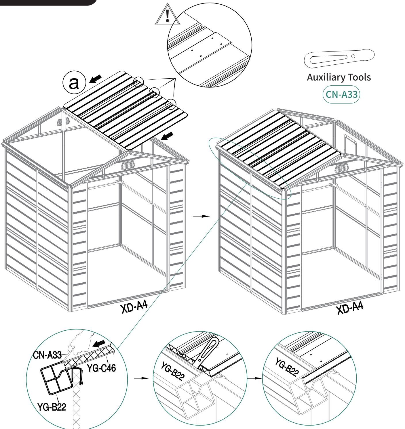
When sliding the roof panels into the slots, please use an assisting tool to ensure they are fully inserted into the tracks.
