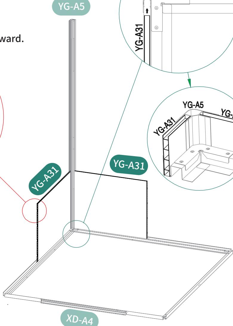
Ensure the panels are fully inserted into the slots to avoid issues with inserting subsequent panels.
