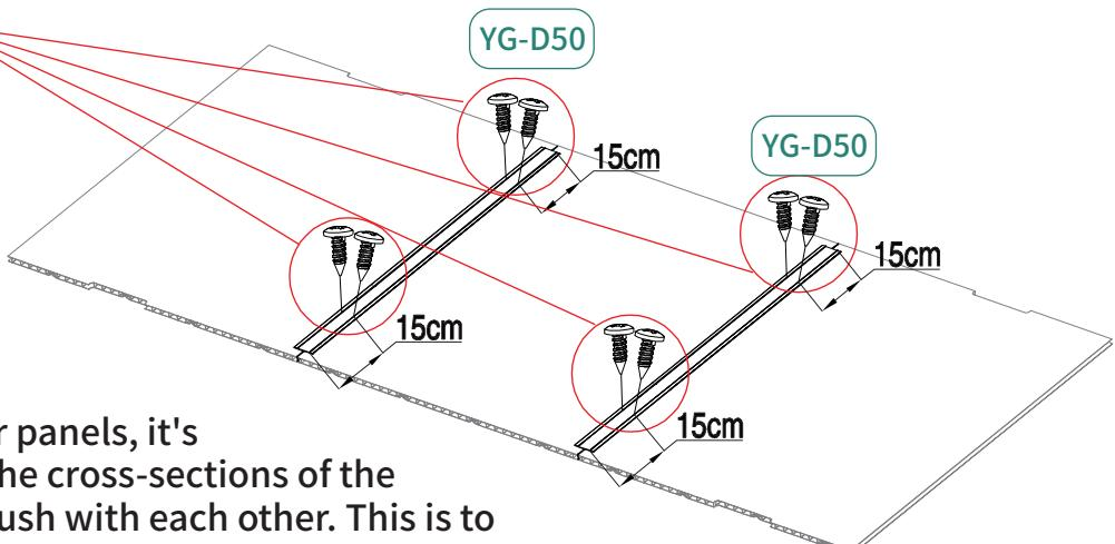
When assembling the door panels, it's important to ensure that the cross-sections of the various components are flush with each other. This is to prevent the door panel from warping after the frame is installed.
