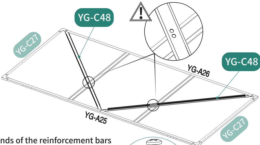
The two ends of the reinforcement bars need to be inserted into the recesses at the bottom of the door threshold. After aligning the holes, secure the bars in place.
