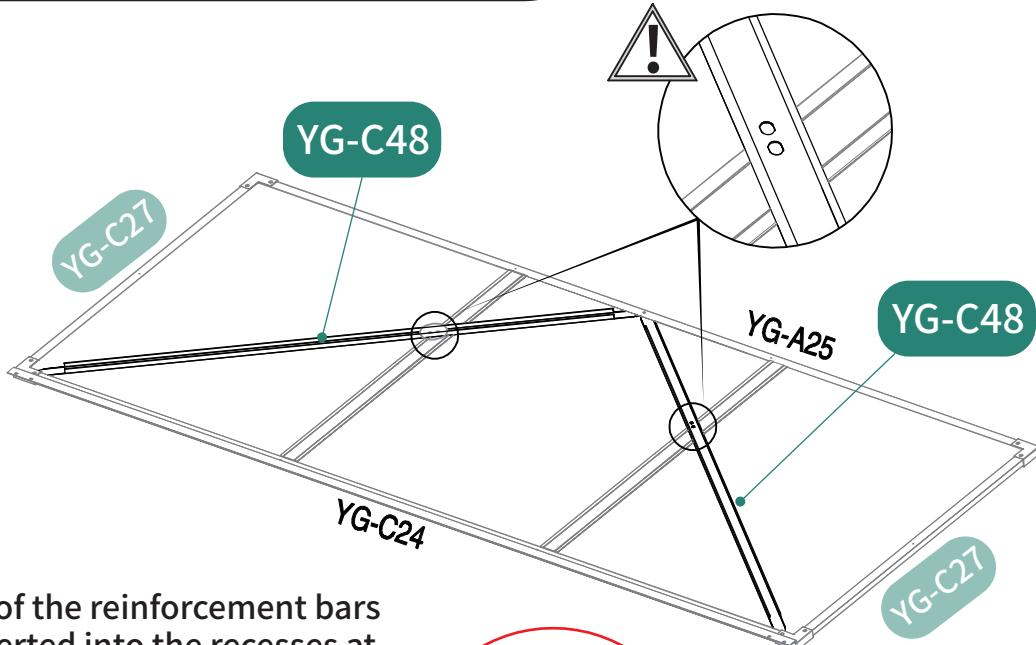
The two ends of the reinforcement bars need to be inserted into the recesses at the bottom of the door threshold. After aligning the holes, secure the bars in place.
