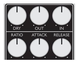
**IN:** This control sets the signal level into the compression circuit, with higher levels resulting in more compression. Like an 1176®, The Cali76 FET Compressor has a fixed threshold (the level above which compression is applied). Increasing the IN control pushes more of your signal over that threshold, meaning that a greater portion of the signal is compressed. Increasing the IN control will also make the signal louder, so this should be balanced with the OUT control.
