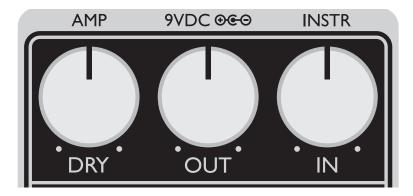
**9VDC:** Connect a 9VDC 2.1 mm centre-negative mains power adaptor (minimum 200mA). Voltage is increased internally for additional headroom.
