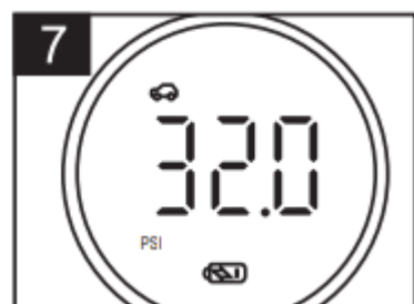
Use the + and - buttons to adjust the target pressure.
