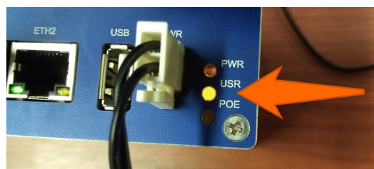
Figure 31: Example 1 – user LED turned on
