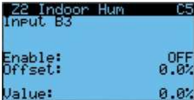
FIGURE 34 Enable/Disable Zone 2 Indoor Humidity Sensor
