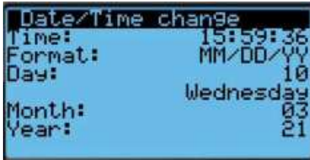
FIGURE 31 Setting Controller Date and Time
