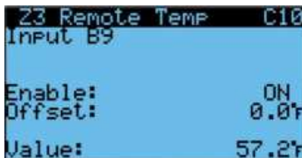
FIGURE 39 Enable/Disable Zone 3 Remote Temperature Sensor
