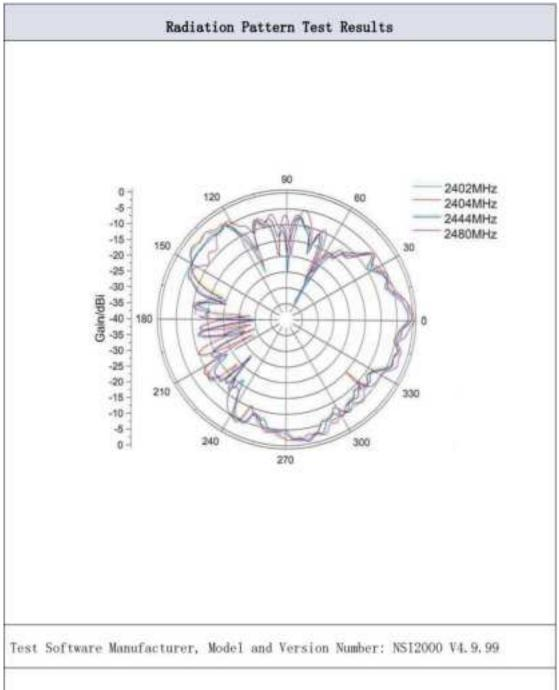
Figure 3. 1-1 Multiple connected self-organizing network communication modules Radiation Pattern Test Curve (AUT Vertical Installation Azimuth Plane 2. 402GHz 2. 404GHz, 2. 444GHz, 2. 480GHz)
