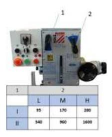
To set a specific speed, move the two levers to the position shown in the table.
