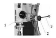
The spindle lift can be moved downwards/up by turning the lever (3). The hand screw (2) is tightened for fine adjustment and the lift can now be finely adjusted to the desired height using the hand wheel (1).
