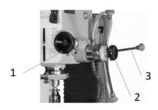
The spindle lift can be moved downwards/up by turning the lever (3). The hand screw (2) is tightened for fine adjustment and the lift can now be finely adjusted to the desired height using the hand wheel (1).
