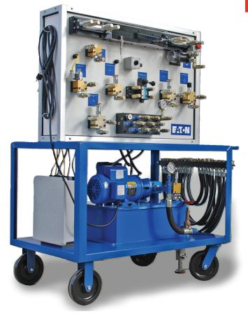
Using the HTS-2, students will become familiar with the principles of aeration and cavitation, sequencing circuits, operation of components in series and parallel, flow control characteristics and types of applications, hydraulically counterbalancing an actuator and many other fundamental concepts.
