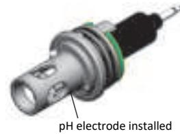
7. Push the sensor end cap back into the logger, making sure the small tab in the end cap fits in the small groove in the logger housing. Use the large tab on the end cap and the arrow on the logger housing to help with proper alignment. Do not twist or turn the end cap as you push it straight into position.
