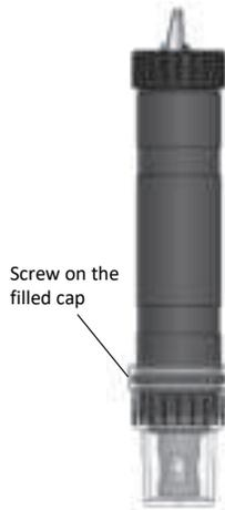
**Important:** Keep the sensor in storage solution unless you are calibrating the logger or deploying it in water. Only use storage solution in the cap; do not use water. Do not use the copper guard while the sensor is in the cap.
