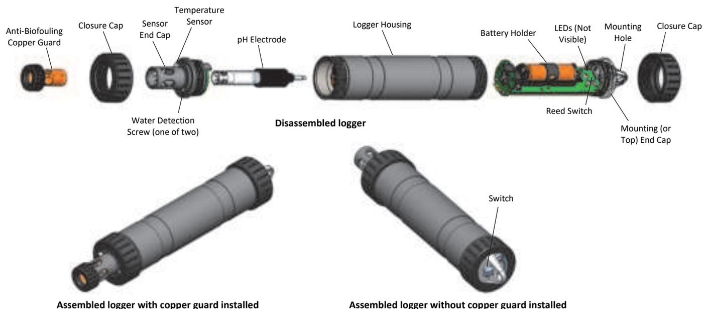
**Anti-Biofouling Copper Guard:** Use this guard to protect the pH electrode when deploying the logger in water prone to biofouling (see *Deploying and Mounting the Logger*).
