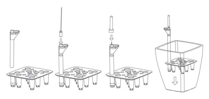
**Step 1:** Secure cylinder to support base
