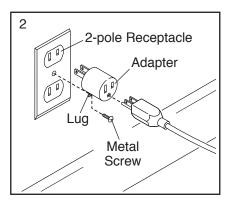
The lug or wire extending from the adapter must be connected with a metal screw to a permanent ground such as a properly grounded outlet box cover. Some 2-pole receptacle outlet box covers are not grounded. Before using an adapter, contact a qualified electrician to determine whether the outlet box cover is grounded. The temporary adapter should be used only until a properly grounded outlet can be installed by a qualified electrician.
