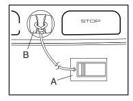
may take some time for the console to be ready for use. IMPORTANT: In an emergency, the key can be pulled from the console, causing the walking belt to slow to a stop. Test the clip by carefully taking a few steps backward; if the key is not pulled from the console, adjust the position of the clip.
