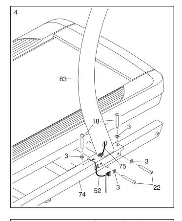
5. See the inset drawing. Connect the Base Wire (52) to the Upright Wire (75). The connectors should slide together easily and snap into place. If they do not, turn one connector and try again. IF YOU DO NOT CONNECT THE CONNECTORS PROPERLY, THE CONSOLE MAY BECOME DAMAGED WHEN YOU TURN ON THE POWER.
