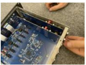
4. Install the I/O Card cover plates with the H035 3/32" Allen screws that were previously removed and H165 3/16" hex standoffs. The H165s will have thread locking compound pre-applied. Place the H591 Dust Cap on the higher slot number card.
