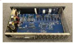
2. Remove the option cover plate(s). The cover plates are held on by two 3/32" Allen screws. Retain these screws for the installation.
