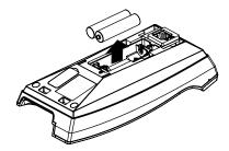
3. Place the new batteries into the battery compartment according to the polarity markings (+/-). Ensure the positive terminal of the battery aligns with the "+" mark in the compartment and the negative terminal with the "-" mark. Follow the markings inside the battery compartment to avoid improper insertion.
