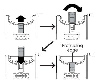
2. Turn the telephone base over with the bottom side facing up. Press the tabs of the mounting bracket as the direction indicated into the grooves on the telephone base until they lock securely.
