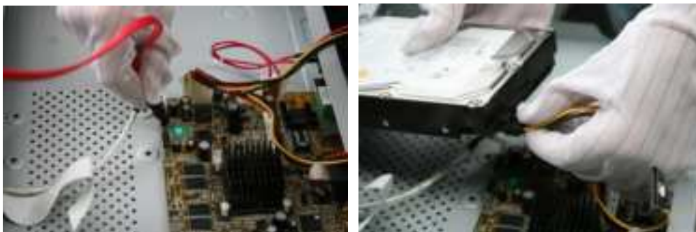
Figure 2-2 Connect Data Cable
