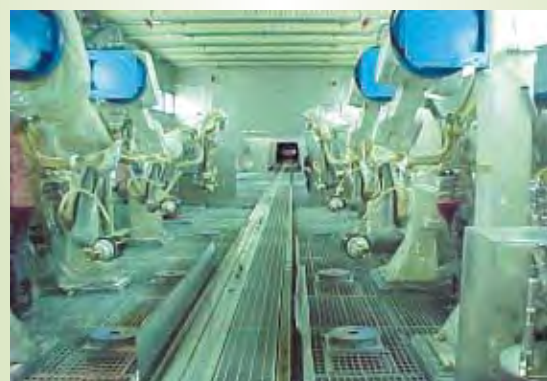
Toyota continues to reduce solvent emissions by installing the latest painting technology, such as this state-of-the-art paint booth.
