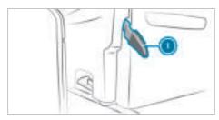
(i) If the seat sliders on the front rear seat row are too far back in the guide rails, the seat/bunk combination cannot be moved forward. In this case, use the handle for the seat sliders to move the seat sliders
