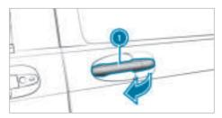
The sliding door is equipped with an active retainer, which engages when the door is opened as far as it will go.
