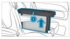
➤ To fold out the table panel: pull out the table panels upwards as far as they will go using handles ② and swing them to the side until they engage.
