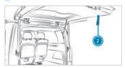
To close: pull the tailgate firmly downwards by loop 2 and close it from outside.
