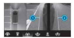
Example: forward-facing side cameras (front wheel view)
