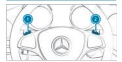
You can change gear manually with the steering wheel gearshift paddles when the automatic transmission is in position  $\boxed{\textbf{D}}$ . If permissible, the automatic transmission shifts to a higher or lower gear depending on the steering wheel gearshift paddle that has been pulled.
