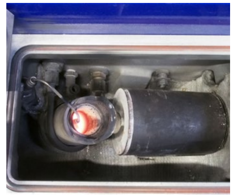
Vacuum or centrifugal casting methods improve fill to thin details.
