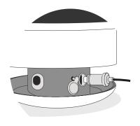
In order for the lights to turn on, the USB plug needs to be inserted into the USB Power Port. Once the plug is inserted, push the power button, and your string lights will shine!
