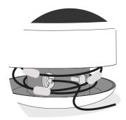
Inside the Power Hub are 2 USB slots (see 10 & 11 above). The USB Storage Slot is for protection of the USB plug when the string is wrapped inside the Power Hub. Storing it in here stops the USB plug from fraying and allows you to wind the string easier.
