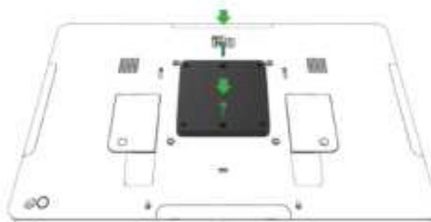
Install optional spacer included if using 100x100mm VESA mount. Place it over the adaptor before adding VESA mounting bracket.
