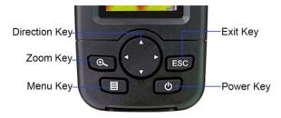
**Power Key** --- Press and hold the power key for 2 seconds, the display unit will power on. The display unit starts working. Press and hold the power key for 3 seconds, the display unit will power off.
