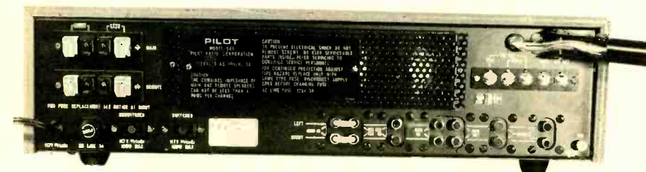
The rear panel of the Pilot 540 with the pivoting AM antenna moved out of the way. Note the jumpers joining the preamplifier and power-amplifier sections and the speaker spring-clips.
