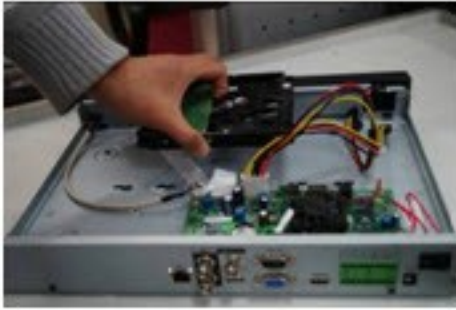
Figure 15-3 Placing the HDD
