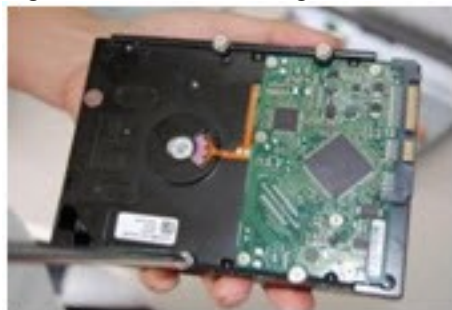
Figure 15-14 Loosening the Four Screws in the HDD Housing
