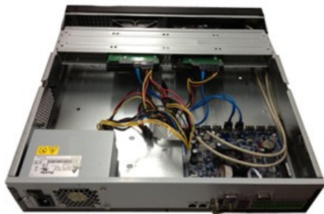
Figure 15-16 Connecting the HDD and the Power Cable
