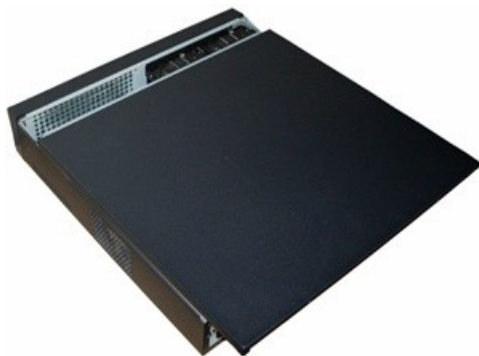
Figure 15-17 Replacing the NVR Cover
