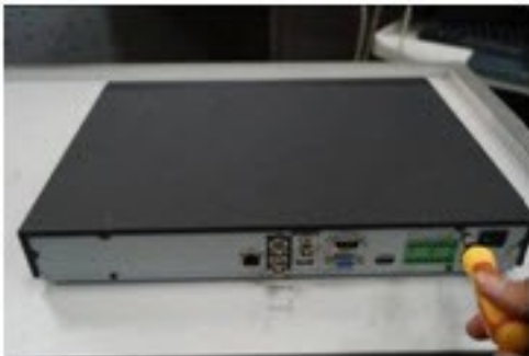
Figure 15-7 Securing the NVR Cover
