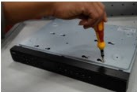
Figure 15-4 Securing the HDD to the NVR Housing
