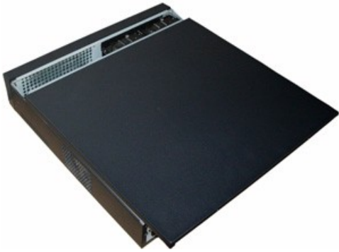
Figure 15-12 Replacing the NVR Cover
