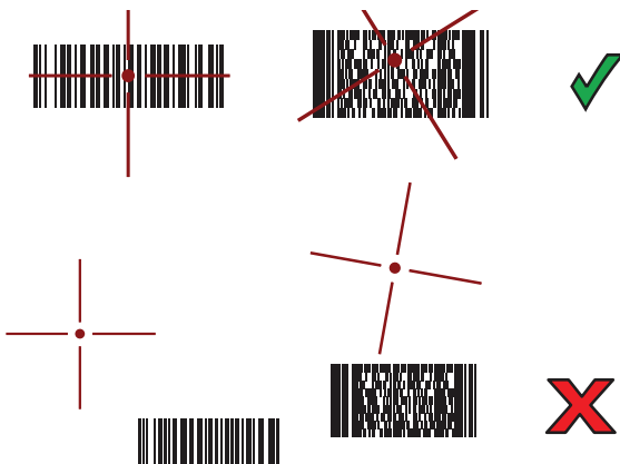
Figure 26 RS5100 Pick List Mode with Multiple Barcodes in Aiming Pattern
