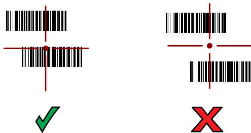
Figure 23 RS6000 Pick List Mode with Multiple Barcodes in Aiming Pattern
