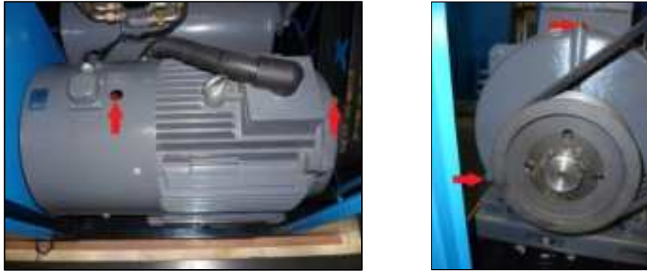
Figure 6-7 Motor Bearing Re-Greasing
