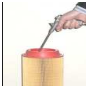
Figure 6-3 Air Filter Element Cleaning
