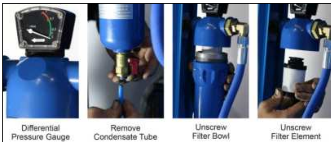
Figure 6-4 Compressed Air Filter Replacement
