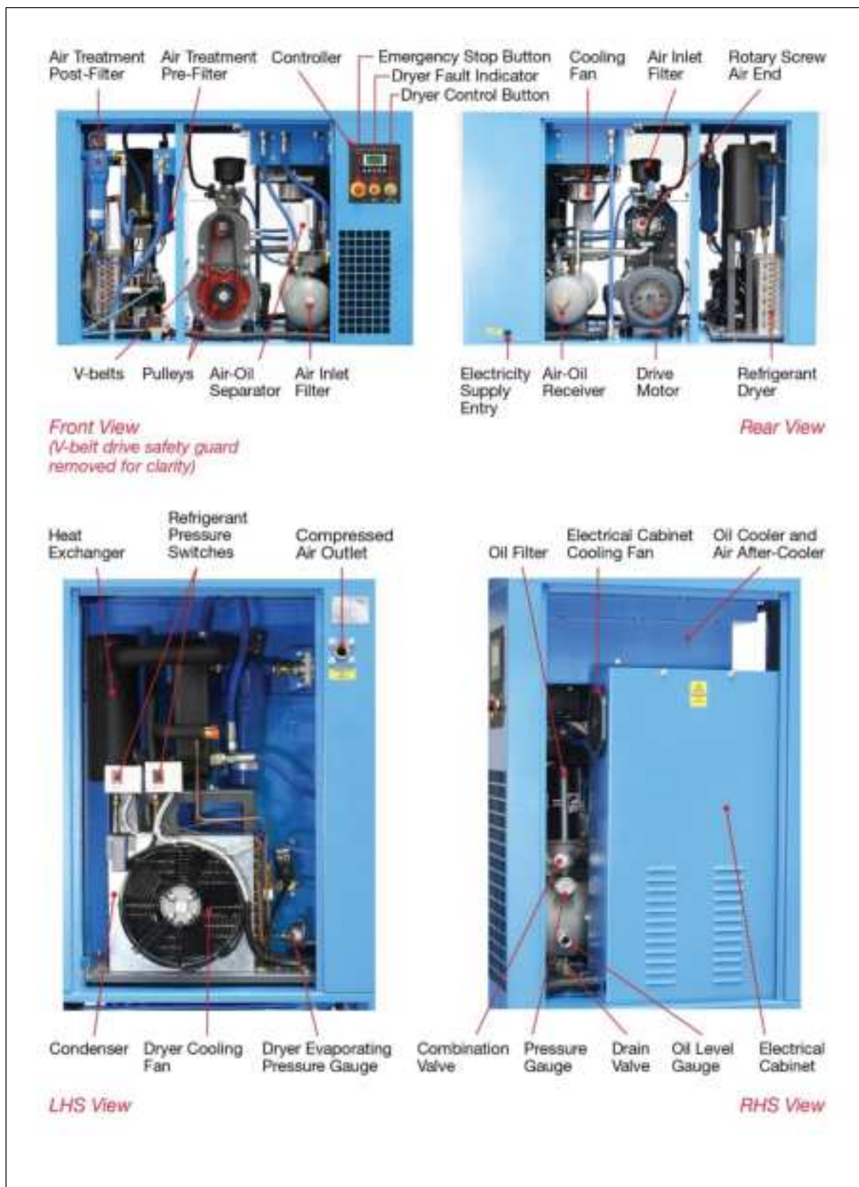
Figure 3-3 Internal Features of CSV Series Air Compressor Set
