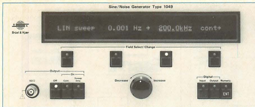
Fig. 5. Vacuum fluorescent line display, plus the field select and speeder controls of the 1049 and 1051
