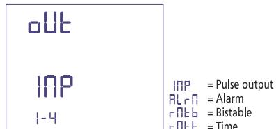
The output relay (terminals 15 - 29) can be used as **energy pulses** (see point 1.7a) repeater or as **alarm relay** (see point 1.7b) or as remote-controlled **state of relay switching** (see point 1.7c - point 1.7c ).
