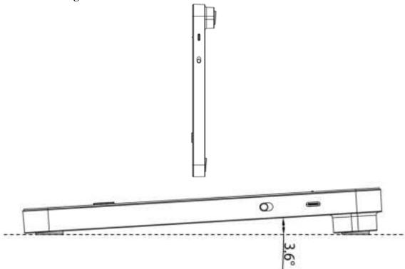
On the right side of the Dot Pad 320, starting from the rear to the front, there is a USB C type power charging port, followed by a power switch. A USB C type power port is a power only port. Keep in mind that there is no option of data transfer from this port.
