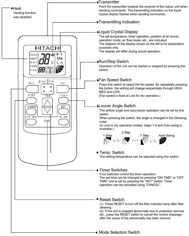
By repeatedly pressing the mode switch, the unit cycles through the different operating modes in order of DRY, COOL and FAN. To select auto operation, press the switch for more than 3 seconds. If the switch is pressed again, it will return to FAN mode.
