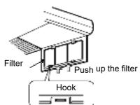
3. Push the filter up, make the filter into a bow shape and remove from the hook. And then pull forward; take out the air filter from the air inlet grille.
