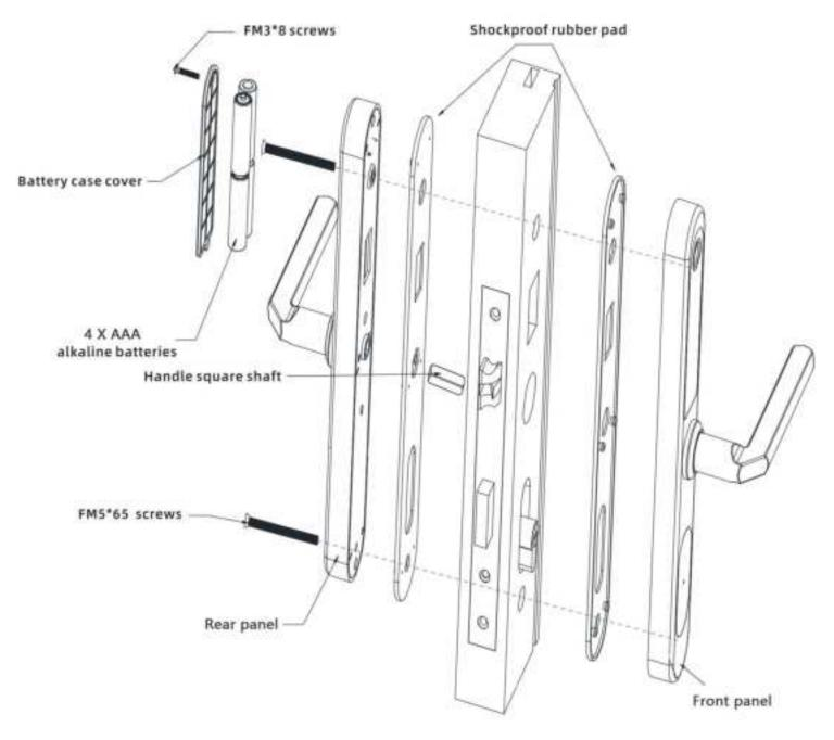
**NOTE**: There is an arrow on the inside of the front panel that needs to face the side of the door opening (Please review the installation video we provide)
