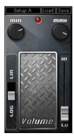
**VOLUME BAR (HI > LO)** controls output level. The position between Hi and Lo determines output volume according to the selected scaling.
