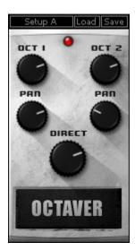
**DIRECT** controls the volume of the direct signal.
