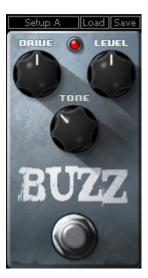
**DRIVE** controls the amount of distortion applied to the signal.
