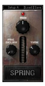
Mix controls the balance between Wet and Dry signal.
