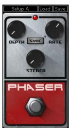
**DEPTH** controls the amount of effect applied to the signal.
