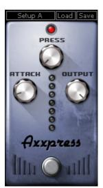
PRESS controls threshold and makeup gain simultaneously.
