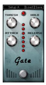
**THRESHOLD** controls the sensitivity of the gate.
