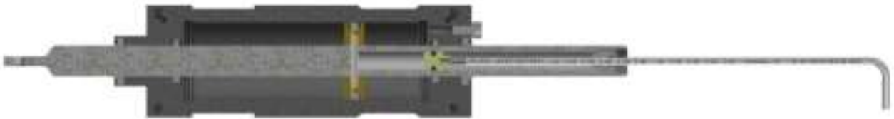
Figure 2: Section View of Fluid Check Procedure
