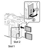
Slot 1 on this camera supports both CFexpress Type A memory cards and SD memory cards, while slot 2 supports only SD memory cards. In the default settings, images are recorded on the memory card in Slot 1. For detailed setup instructions, refer to the Help Guide. When you use a memory card with the camera for the first time, it is recommended that you format the card on the camera for more stable performance of the memory card.
