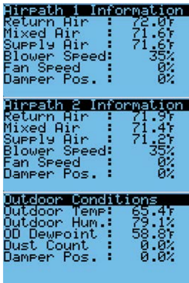
FIGURE 6 Unit Air Path Information
