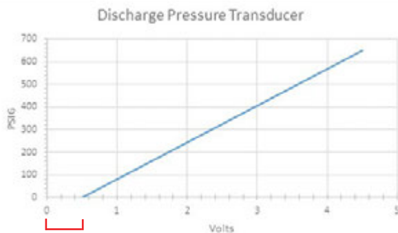
FIGURE 40 Voltage to Pressure: Discharge/Liquid Pressure Transducer
