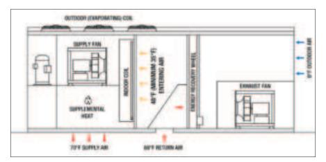
If a recirculation damper is not available, an enthalpy wheel and/or preheat coil may be able to deliver the necessary air temperatures during these periods. Optimizing the unit design efficiency by pairing energy recovery with a high outdoor air ASHP can help avoid this low-temperature issue and reduce energy consumption. Energy recovery devices temper incoming air using previously heated return/exhaust air, thus ensuring the incoming air is warm enough when it reaches the indoor coil.
