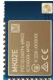
MK02E u.FL Connector 21.0x13.8x2.3mm
