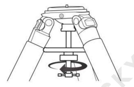
Fix the silver connection plate of the tripod to the bottom of UMi 17R with three M6\*10 screws as shown below:
