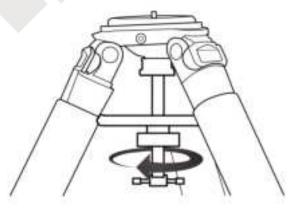
Fix the silver connection plate of the tripod to the bottom of PE149 with
